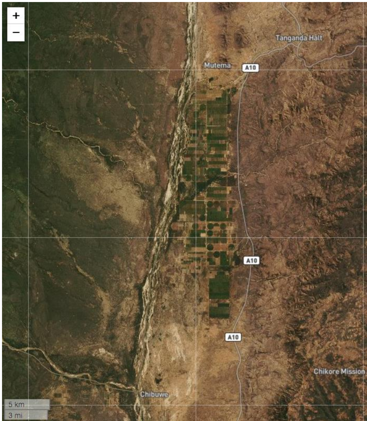
Figure 47: Middle Save alluvial aquifer \pm 15,000 ha. Water pumped from the alluvial aquifer is recharged by river flow at the expense of downstream river discharge.
