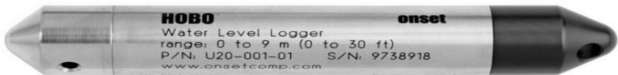
Figure 75: Automatic water-level recorder. These devices work with a pressure transducer that senses the height/head of the overlying water column. They also may have other sensors such as EC and T.
