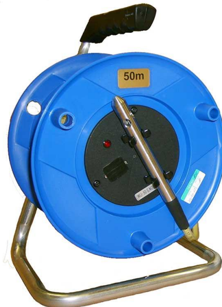
Figure 74: Dip meter. Dip meters come with different length of tape, typically 30m, 50m and 100m. It is also possible to get manual dip-meters that have EC (electrical conductivity) and T (temperature) sensors. The tape on dippers can become snagged down the borehole quite easily and it is recommended to insert a 25mm PVC tube down the borehole as a dipper access tube.
