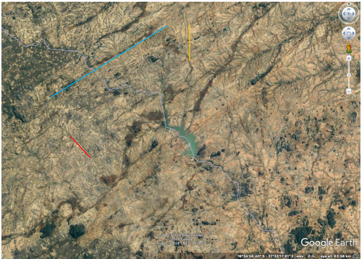
Figure 25: Granitic crystalline basement. The lineaments are readily visible as “lines” on the image. Some of these lines represent straight river reaches (e.g. NE corner of the image); other lines, especially those oriented NE (blue line) are dykes. Fractures and fracture intersections are generally good for groundwater. Regional principal compressive stress is NE-SW oriented and therefore the NW fractures (red line) are under compression, while the NE fractures (blue line) are under dilation and tend to be most productive for groundwater (Image scale approximately 50 km x 80 km).
